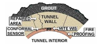
Figure 2. MITE WIS Installed in Tunnel
