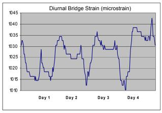
Strains produced by diurnal heating
