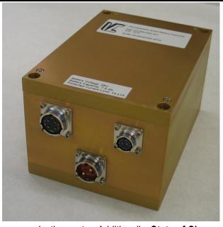
measures key battery parameters and provides this information on communication ports. Additionally, **State of Charge** (SOC) and **State of Health (SOH)** are continuously calculated so you always know the condition of the batteries in order to insure sufficient mission power and reliability.
