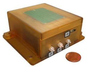
The Enhanced Wide-Band Microminiature Tri-Axial Accelerometer Unit (EWB MicroTAU) system is a wireless, high-speed, synchronized data acquisition network for dynamic acceleration sensing, processing, and recording applications. The system includes EWB MicroTAU Remote Units, a EWB MicroTAU Receiver Unit, and the Graphical User Interface (GUI).
