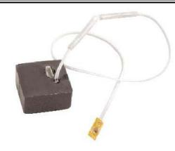
MicroRecorder is a data acquisition unit that measures and stores data for post-acquisition download to a PC. Over one month of data (at one sample per minute) can be recorded on internal non-volatile memory. Each unit has one external input channel from a resistive sensor and an internal temperature channel. Each unit has a programmable acquisition initiation time and programmable sample rate.
