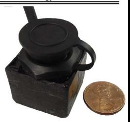
acquisition and processing for programmable periods up to 23 hours 59 minutes. The schedule also dictates the low-power sleep time between active modes; sleep modes are also programmable from one minute to one week. Over one year of processed data can be stored in the unit in non-volatile memory. The Rainflow processing has programmable strain ranges for the 32 bins that count the total excursion cycles.
