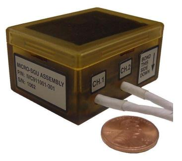
The MicroSGU system was designed for NASA and successfully flown on the Shuttle since 2001 to detect strain of components during launch. Other applications where the triggered initiation capability may be appropriate are railroads, bridges, industrial equipment, and other structures or components that experience random stresses.
