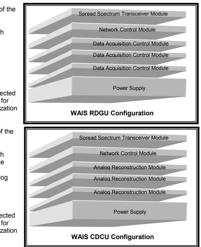
The CDCU is the system link to the Graphical User Interface. All front-end setup parameters and network timing constraints are generated by the GUI with system user input and subsequently sent to the CDCU. The CDCU is the network activity controller. Setup parameters are automatically sent via RF to the appropriate node. Once the setup is complete, the system is ready for operation. The following is a listing of some functions available using the GUI:
