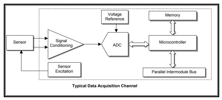
Each Data Acquisition Module utilizes a microcontroller to handle data buffering, and parallel communications with the Network Control Module (NCM).
