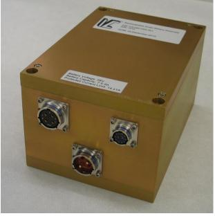
calculated so you always know the condition of the batteries in order to insure sufficient mission power and reliability. Custom circuitry offers options for uninterruptable power discharge for mission critical applications (such as RCC 319 flight termination systems), or prevent further battery discharge under high temperature, undervoltage, and high current conditions.
